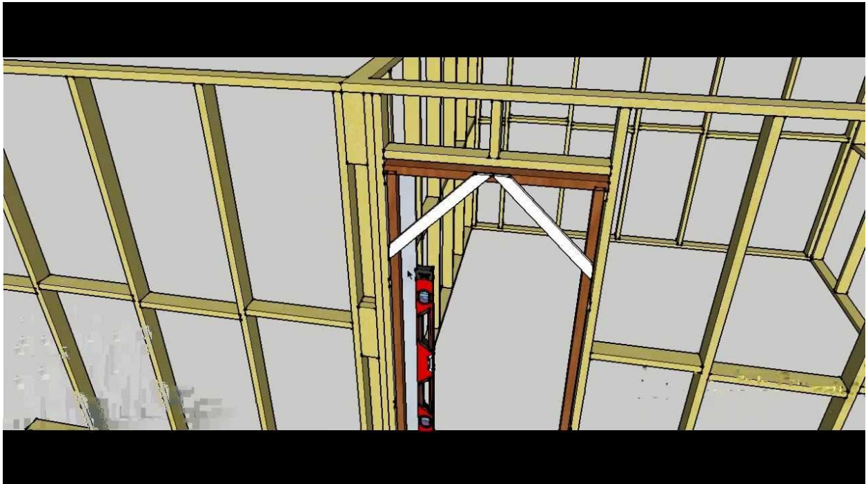
Figure 4 Assembling, squaring and bracing Jamb frame
